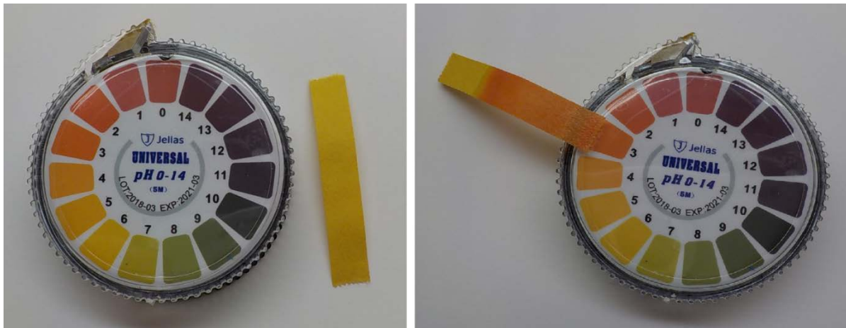
Left: pH test kit litmus paper. Right: Litmus paper after being dipped into the sample.
